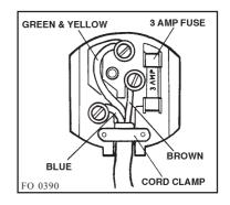
3) Connect the brown (live) wire to the terminal in the plug which is marked with the letter 'L' or coloured red.
